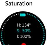
Press Select Button + Rotate Dial to adjust saturation
