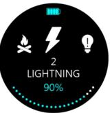
Press Select Button + Rotate Dial to adjust brightness
