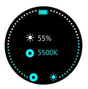
Press Select Button + Rotate Dial to adjust color temperature
