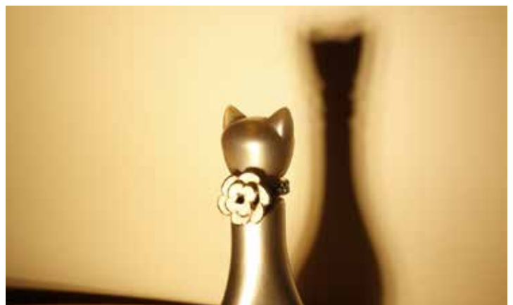
Multi-LED - Light effect on object is blurry and unclear with double images.
